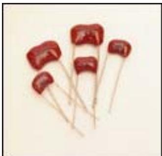
Those caps have a typical "hump" in the middle of the body and can be found inside high-quality amps and stompboxes. They can also be used as a hi-cut cap on the volume pot and if you can find the correct value as a cap for the tone control. Higher values are often hard to find and very expensive.
