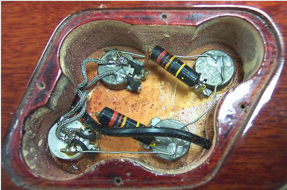
You can often find guitars with a very lousy inside-wiring and cheap parts, crappy soldering spots, weak cables, ultracheap caps and other things seem to be common these days. All this can affect your sound and the reliability of your guitar in a very negative way, so it's worth the time to take care of this.
